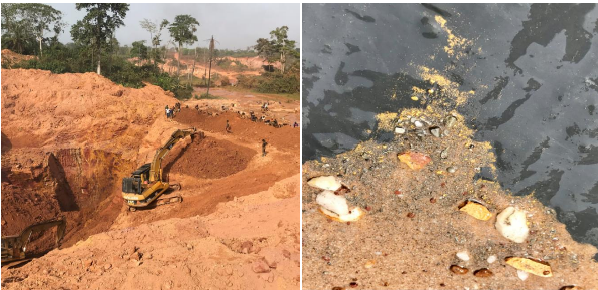
Figure 3: Artisanal workings within the license area and visible gold observed in a washing pan.
